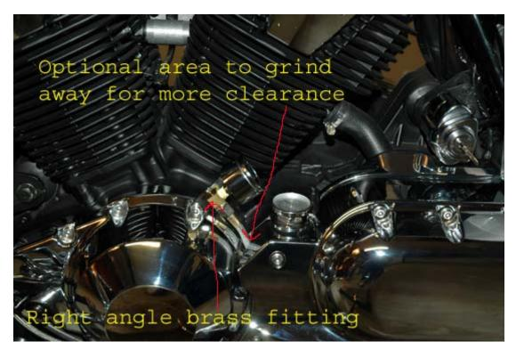
There are two oil gallery bolts under the bike on each side. Since I had the 3' stainless braided cable it allowed me to use the one on the right side of the bike instead of the one on the left side (near the drain plug). The reason I opted for the right side is the left side is harder to get at the bolt due to the chrome cooling line.
