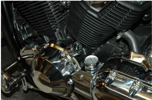
As I mentioned on the web page, making sure that you will not have any problems after this install is crucial since the oil pressure line runs under your bike. A leaky oil line under your bike can have disastrous consequences—mainly because you won't know it's leaking until your bike either runs out of oil or you crash—or both. Remember, it's pumping at around 75 PSI which is like having a gash in your femoral artery; if it springs a leak—you won't last long.
