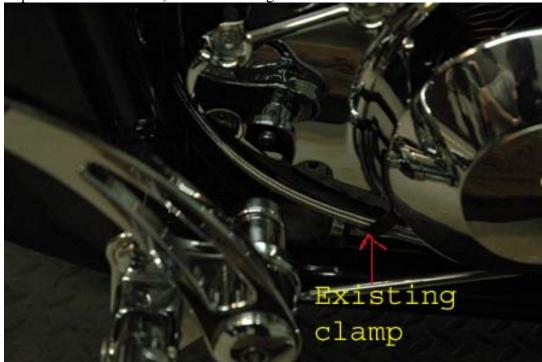
I ran the cable under the bike and fastened it to an already existing clamp on the left side frame which holds a wiring harness.
