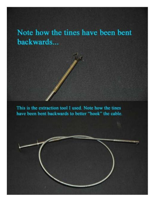
Before you proceed, practice using the extractor tool to see how little you need depress the handle before the claws start to open. Remember—there are burrs from the weld in there and if you open the claws to much you'll just catch on the weld, not the cable.
